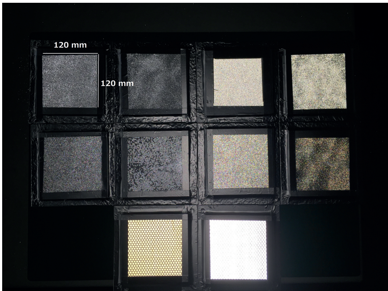
Figure 10. Retroreflection effect of developed glass bead RR materials when the artificial light source is incident on their surface.
