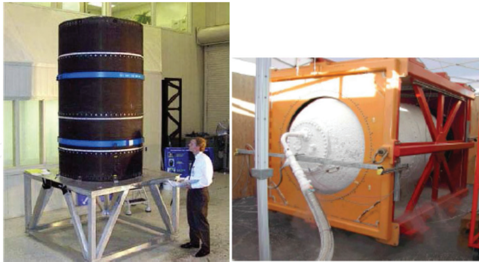
Composite LOx tank Composite LOx tank testing
