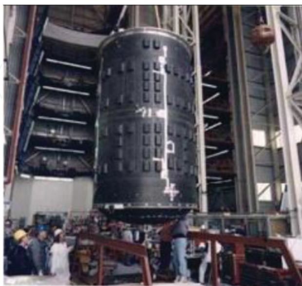
Figure 2. DC-XA composite LH2 cryotank.
