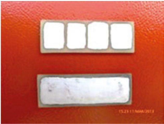
Figure 15. The low energy source built with piezoelectric linear transducers system, INCDIE ICPE-CA concept [26].
