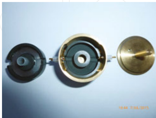
Figure 24. The ferrite magnetic circuit and microtransformer housing.
