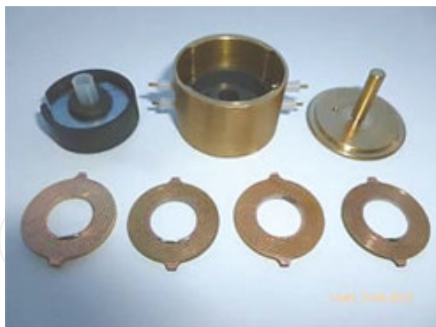
Figure 25. Parts of the housing, the ferrite magnetic circuit and the four planar coils which form the primary and the secondary circuit of the microtransformer, INCDIE ICPE-CA concept [33].
