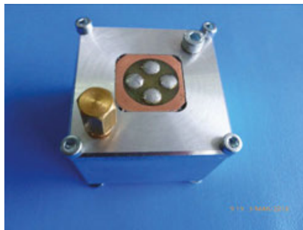
Figure 36. The planar microtransformer with circular spiral windings with hybrid core—ferrite and colloidal magnetic nanofluid, practical achievements.
