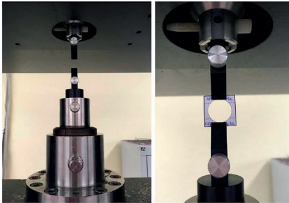
Figure 6. Single fiber disposition in the dynamometer MTS.
