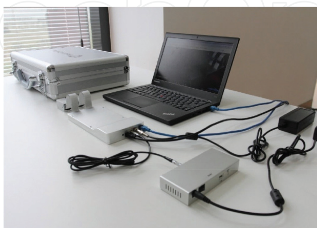
Figure 16. Plug & Imaging PET detector: the mounted system with software chain.
