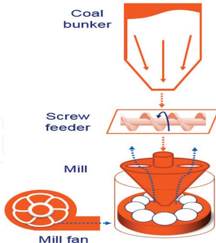
**Figure 1.** Coal mill scheme.
