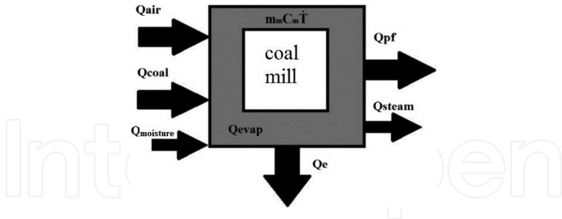
Figure 5. Scheme of coal mill heat balance.
