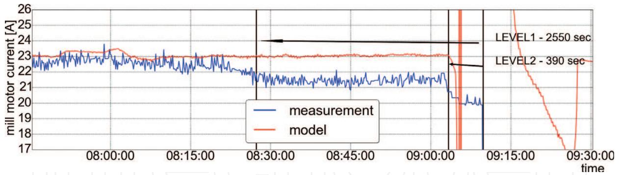
Figure 15. AMPS11 September 2014 fault: Screw blockage.
