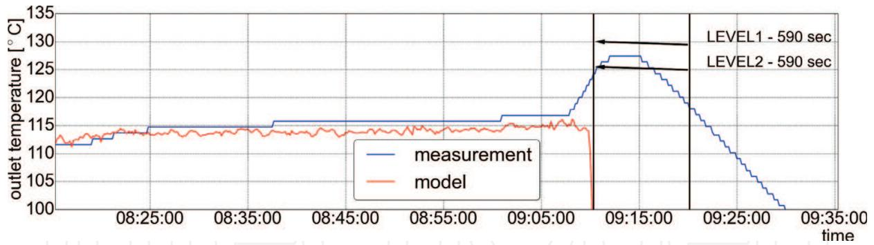
Figure 20. MILL\_OUT\_TEMP 22 January 2014. Fault: Screw blockage.
