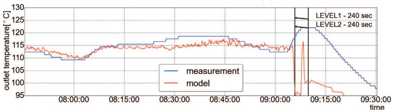
Figure 16. MILL\_OUT\_TEMP 2014.09.11 fault: Screw blockage.
