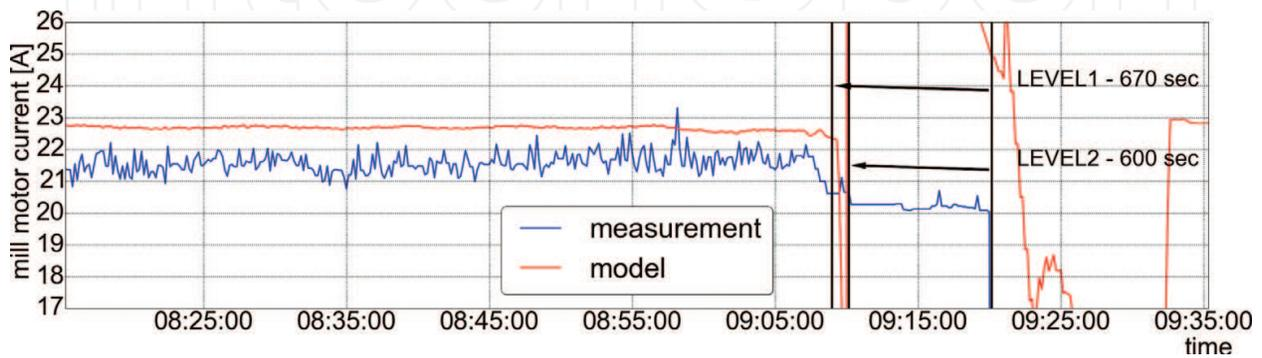
Figure 19. AMPS 22 January 2014. Fault: Screw blockage.
