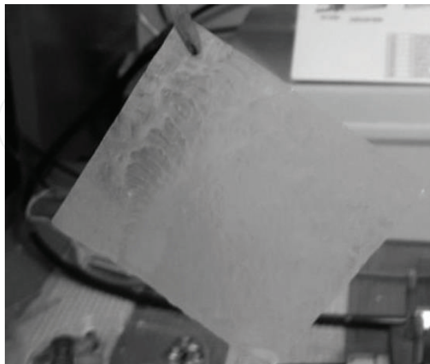
Figure 5. Image of Naf-MOF 801 composite membrane obtained from the sol-gel casting process.
