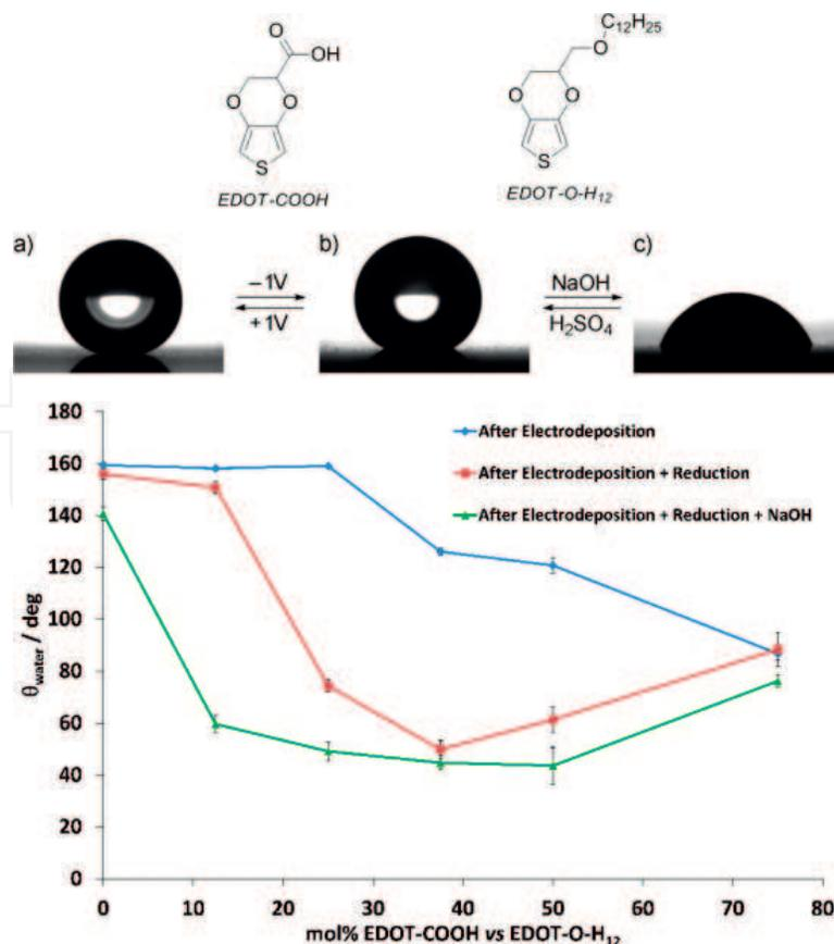
**Figure 18.** Voltage and pH-switchable surfaces using PEDOT-COOH and PEDOT-O-H<sub>12</sub> copolymers [101].
