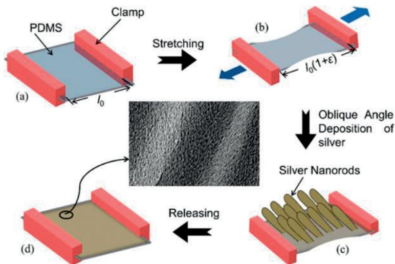
**Figure 7.** Preparation of microwrinkles of PDMS by pre-stretching following by oblique angle deposition of Ag nanorod. Ref. [46], Copyright 2015. Reprinted with permission from American Chemical Society, USA.
