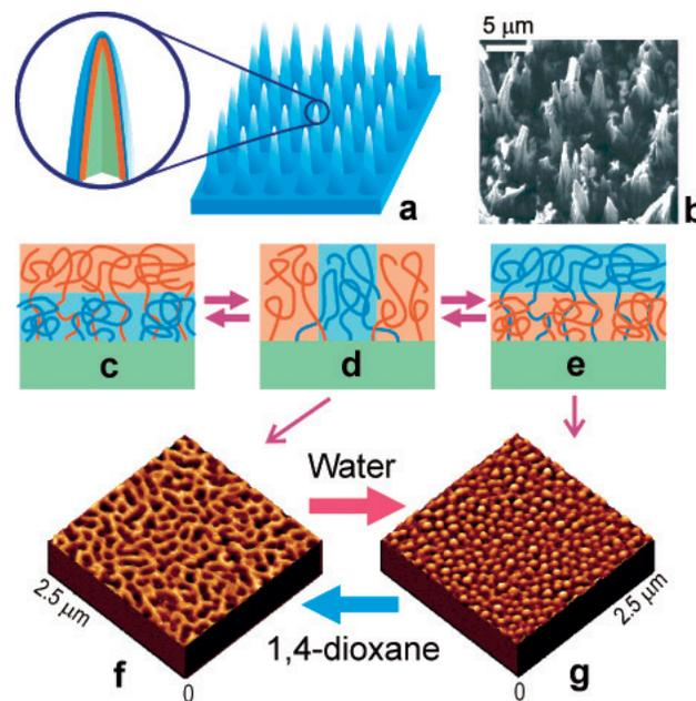
**Figure 10.** Change in the surface topography and organization of needle-like PTFE nanostructures grafted with PSF-COOH and PVP-COOH after exposure to different solvents. Ref. [70], Copyright 2003. Reprinted with permission from American Chemical Society, USA.
