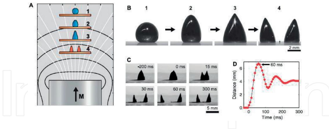
**Figure 5.** Modification of the speed, the shape and the self-assembly of magnetic droplets on the superhydrophobic surface by modulating the magnetic field. Ref. [38], Copyright 2013. Reprinted with permission from The American Association for the Advancement of Science, United Kingdom.
