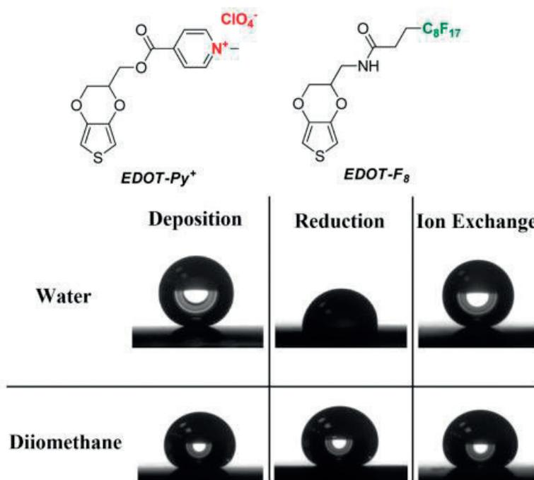
**Figure 19.** Voltage and ion exchange-switchable surfaces using PEDOT-Py<sup>+</sup> and PEDOT-F<sub>8</sub> copolymers [104].
