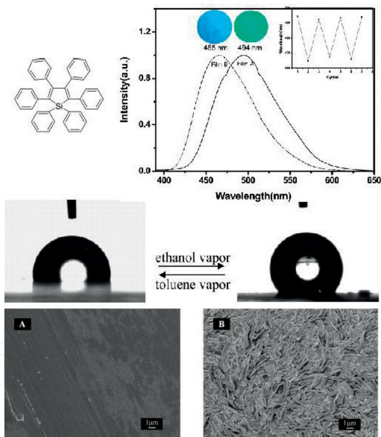
**Figure 12.** Reversible control in the surface structuration, hydrophobicity, and luminescence properties of 1,2,3,4,5-hexaphenylsilole films after exposure to ethanol vapor and toluene vapor, respectively. Ref. [74], Copyright 2008. Reprinted with permission from American Chemical Society, USA.
