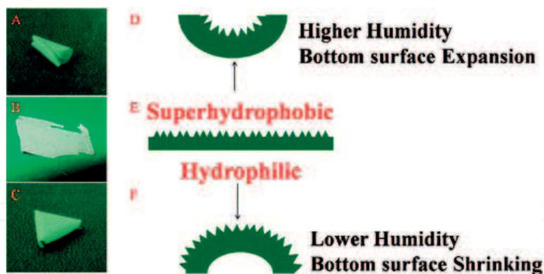
**Figure 11.** Control in the bending of free-standing films prepared by LbL of PEI and PAA as a function of humidity. Ref. [71], Copyright 2010. Reprinted with permission from American Chemical Society, USA.
