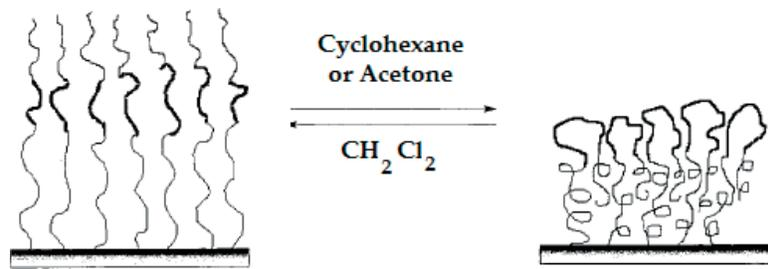
**Figure 9.** Changing in the organization of mixed polymer brushes with hydrophobic and hydrophilic blocks after exposure to different solvents. Ref. [63], Copyright 2002. Reprinted with permission from American Chemical Society, USA.
