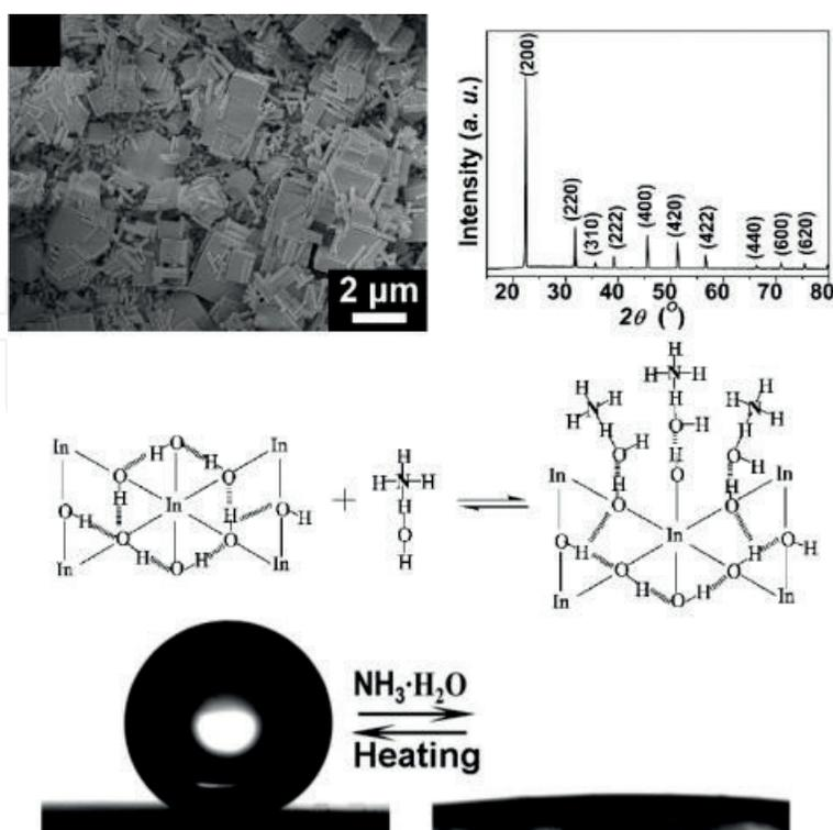
**Figure 13.** Influence of  $\text{NH}_3 \cdot \text{H}_2\text{O}$  on the surface hydrophobicity of  $\text{In}(\text{OH})_3$  with microcubes and nanorods. Ref. [80], Copyright 2008. Reprinted with permission from American Chemical Society, USA.
