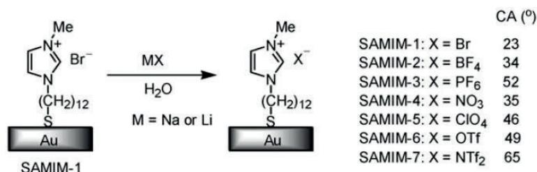
**Figure 1.** Grafting of monolayers on smooth gold substrates with imidazolium groups with sensitivity to ion exchange and surfaced hydrophobicity as a function of the ion-exchanged. Ref. [1], Copyright 2004. Reprinted with permission from American Chemical Society, USA.
