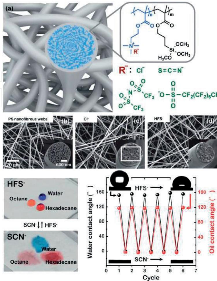
**Figure 3.** Membranes sensitivity to ion exchange prepared by electrospinning of PMETAC-co-TSPM. The resulting membranes could switch from superhydrophobic/highly oleophobic to superhydrophilic/superoleophobic by changing the counter-ions. Ref. [20], copyright 2012. Reprinted with permission from Royal Society of Chemistry, United Kingdom.
