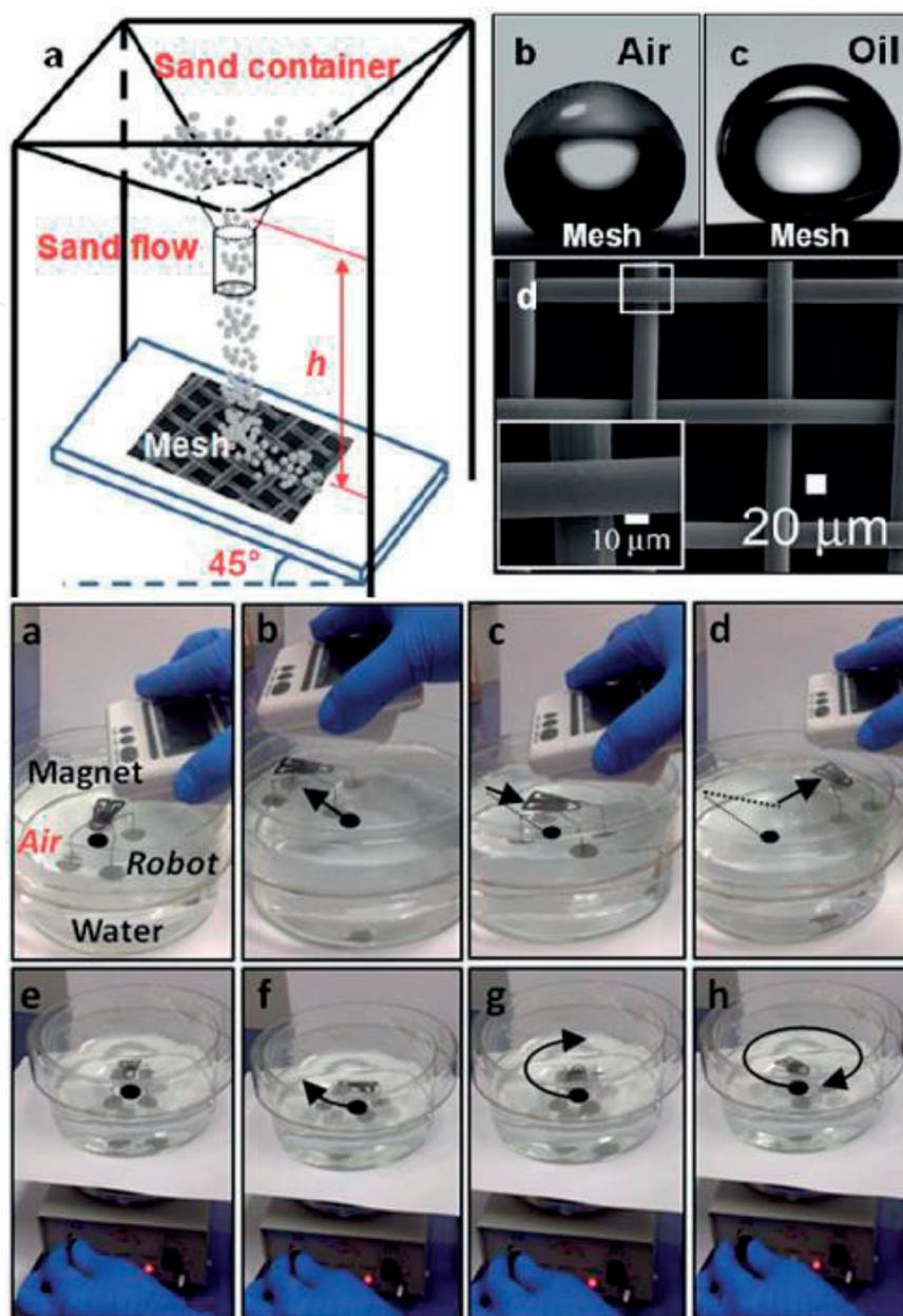
**Figure 4.** Fabrication of micro-robots using magnetically responsive mesh substrates and  $\text{Fe}_3\text{O}_4$  nanoparticles. Ref. [30], Copyright 2015. Reprinted with permission from Royal Society of Chemistry, United Kingdom.
