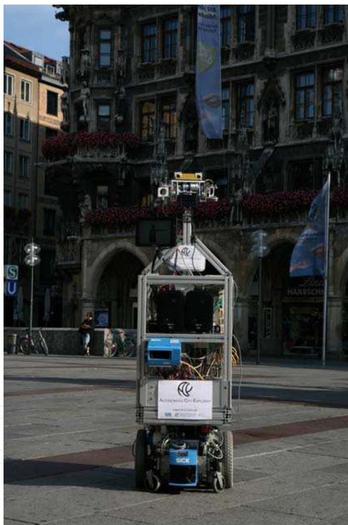
Fig. 1. The Autonomous City Explorer (ACE) robotic platform
