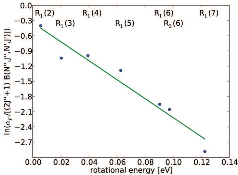
**Figure 9.** Fluorescence gains obtained from probing different absorption lines show Boltzmann distribution corresponding to rotational temperature  $T = (620 \pm 9)$  K.  $J''$  is the quantum number of the probed lower state and  $B$  is the absorption coefficient of the transition. Reprinted from [14] ©IOP publishing. Reproduced with permission. All rights reserved.
