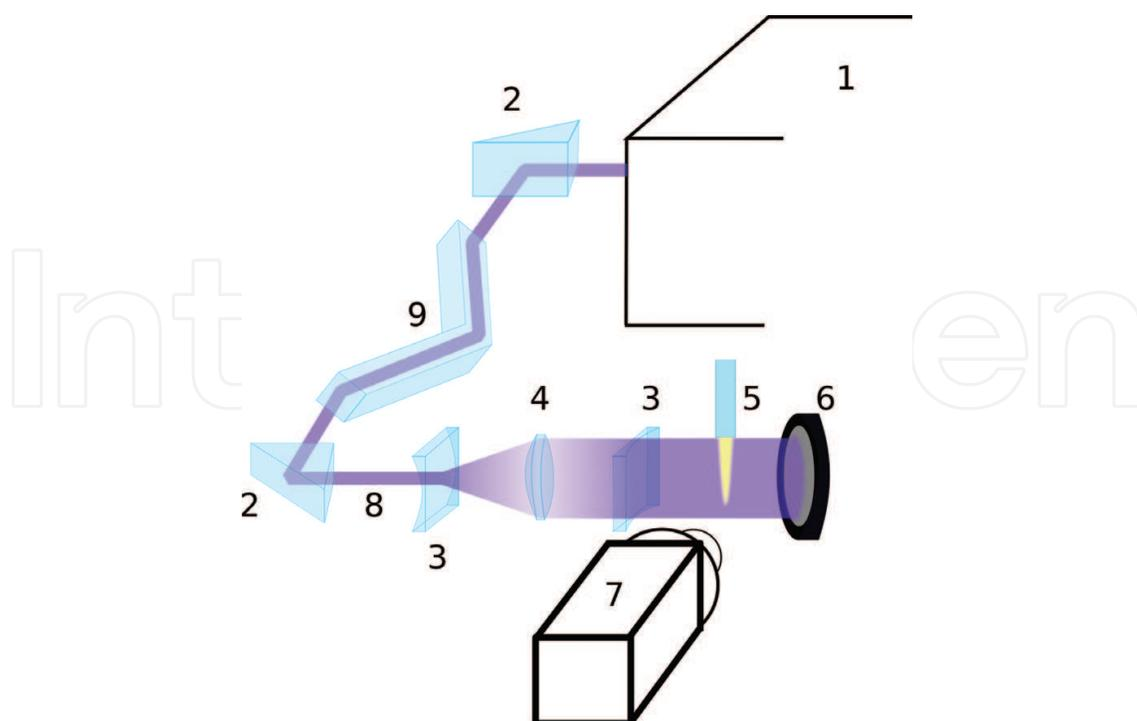
**Figure 5.** Instrumentation of a planar LIF experiment. 1 – Pulsed tunable laser, 2 – Right-angle prism, 3 – Cylindrical negative UV lens, 4 – Spherical positive UV lens, 5 – Investigated plasma source, 6 – Laser-power meter, 7 – ICCD camera synchronized with the laser, 8 – Laser beam, 9 – Fresnel rhomb tandem to turn polarization (if necessary). Reprinted from [14] ©IOP publishing. Reproduced with permission. All rights reserved.
