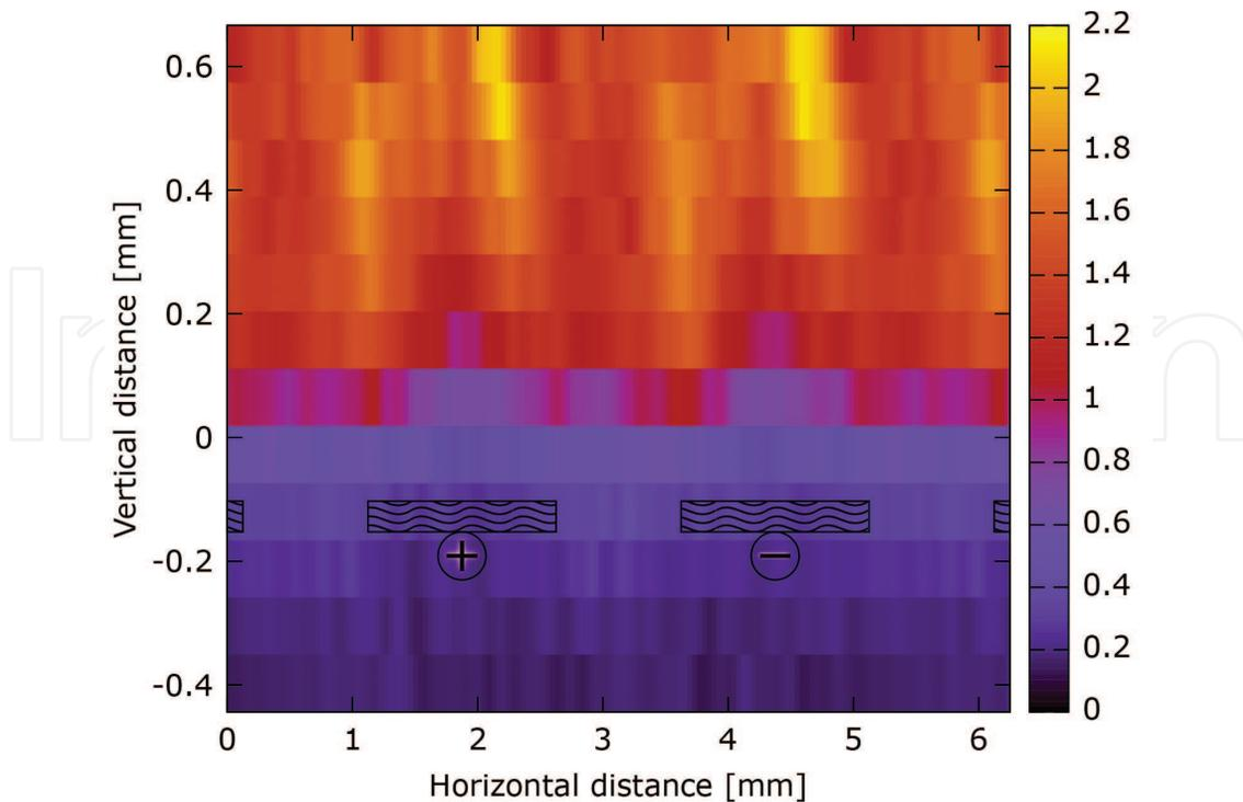
**Figure 15.** Laser radiation scattered on water droplets that were present in the coplanar DBD ignited in water vapor. Measured with laser wavelength detuned from the absorption line of OH radicals. Reprinted from [33] ©IOP publishing. Reproduced with permission. All rights reserved.
