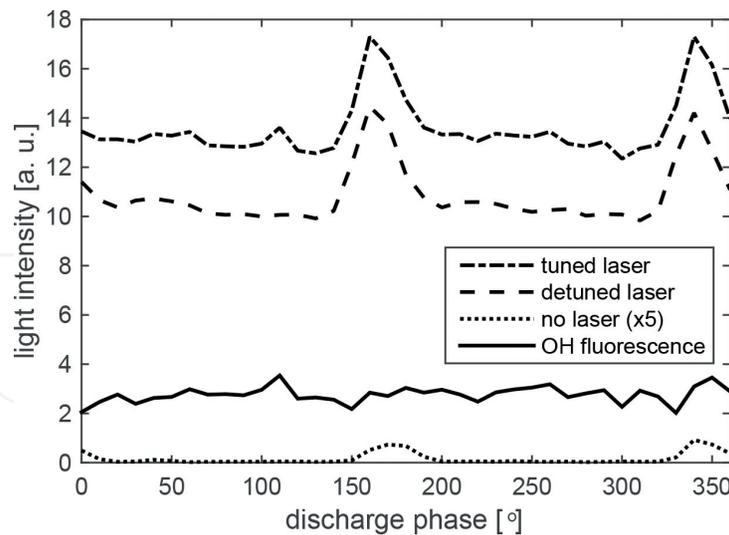
**Figure 6.** Signal strength vs. discharge phase. Dotted line was measured without laser radiation and is magnified 5 $\times$ . Dash-dotted line is with the laser tuned to the OH absorption line, dashed line is with laser detuned. The solid line is the difference between the dash-dotted and the dashed.
