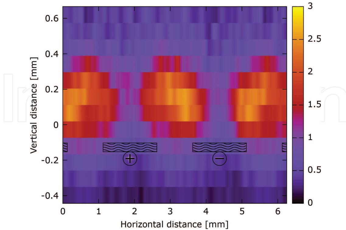
**Figure 16.** Emission of DBD ignited in water vapor at atmospheric pressure. Discharge ignition was synchronized with ICCD measurement by a laser shot. Reprinted from [33] ©IOP publishing. Reproduced with permission. All rights reserved.
