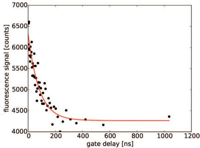
**Figure 11.** An example of the single exponential fit to the measured decay of the fluorescence signal at one pixel for RF driving power of 80 W and argon flow rate of 0.6 slm. The fitted lifetime is  $\tau = (81 \pm 10)$  ns. Reprinted from [14] ©IOP publishing. Reproduced with permission. All rights reserved.
