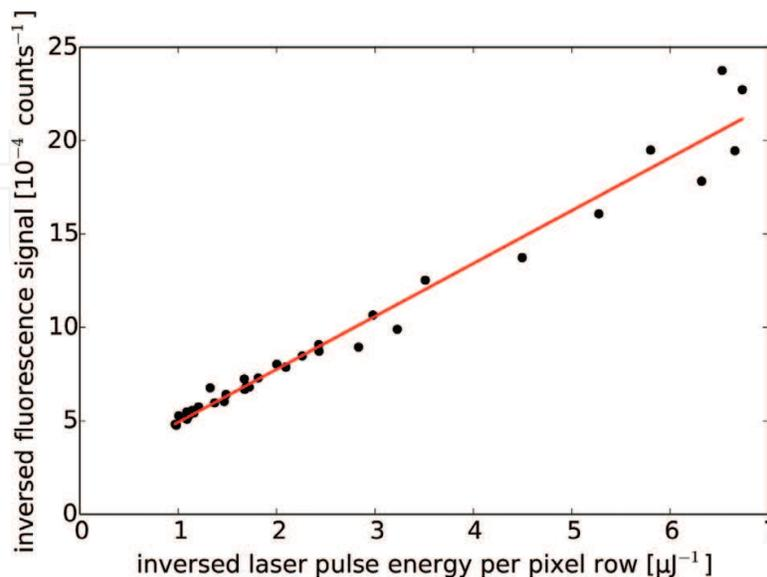
**Figure 8.** An example of the fluorescence gain determination. In the shown case, the fluorescence gain  $\alpha = (3500 \pm 100)$  counts/ $\mu$ .
