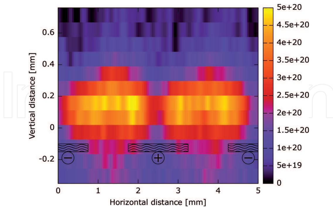
**Figure 17.** OH concentration determined by fluorescence measurement in the coplanar DBD ignited in water vapor at atmospheric pressure. Reprinted from [33] ©IOP publishing. Reproduced with permission. All rights reserved.
