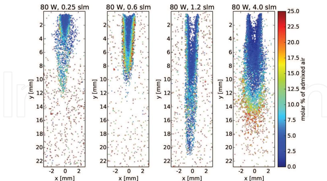
**Figure 12.** Maps of molar percent of ambient air admixed into the argon effluent of the plasma pencil for various conditions. The points with fluorescence lifetime uncertainty greater than 25% are displayed as white. Reprinted from [14] ©IOP publishing. Reproduced with permission. All rights reserved.
