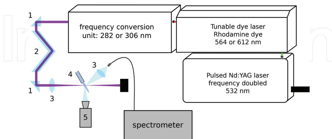
**Figure 4.** Instrumentation of an LIF experiment. 1 – Right-angle prism, 2 – Fresnel rhomb tandem to turn polarization (only, if necessary), 3 – Spherical positive UV lens, 4 – Investigated plasma source, 5 – ICCD camera synchronized with the laser.
