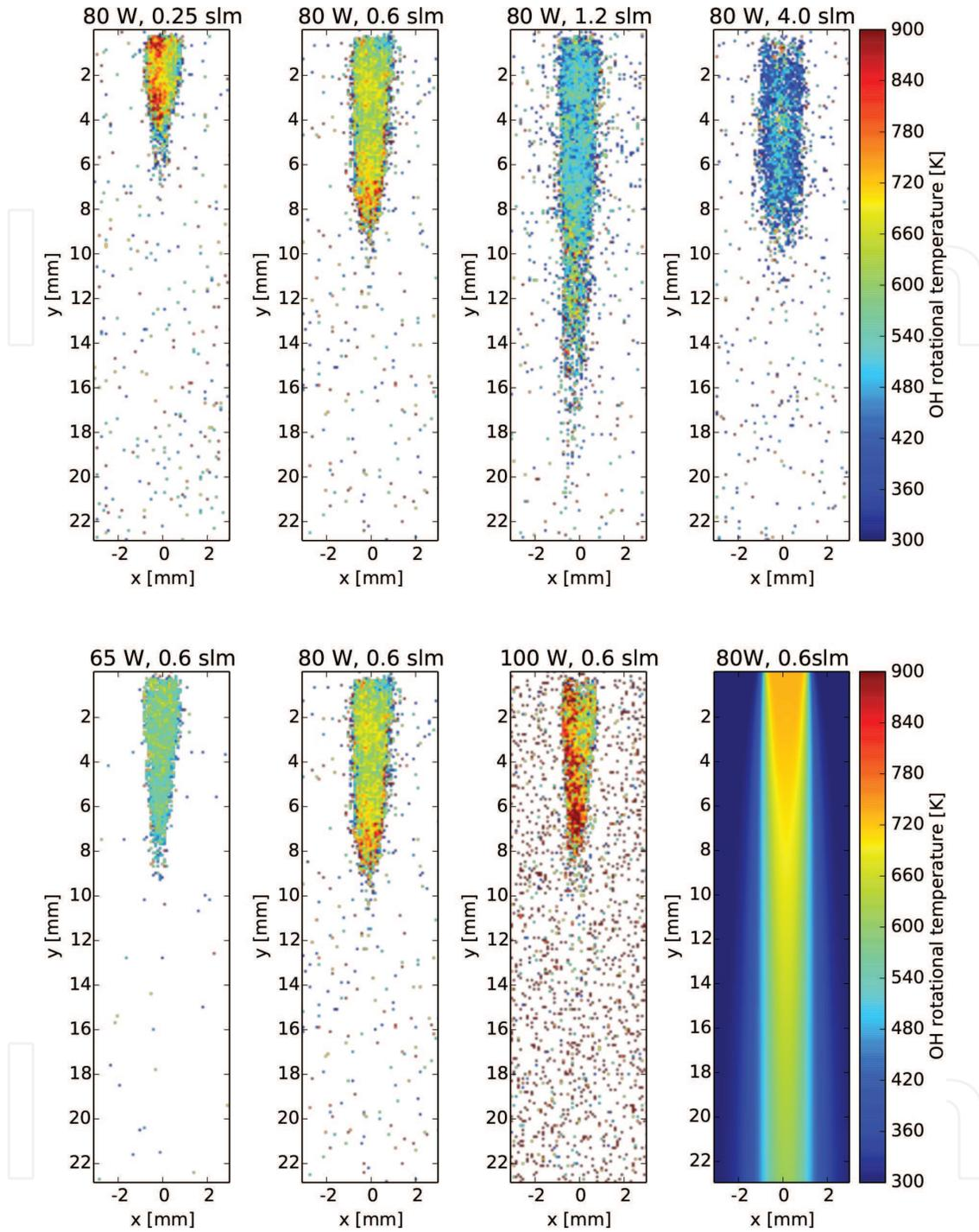
**Figure 10.** Measured discharge temperature for various discharge conditions. Bottom-right: Result of gas dynamics simulation (no plasma taken into account) for comparison. Reprinted from [14] © IOP publishing. Reproduced with permission. All rights reserved.
