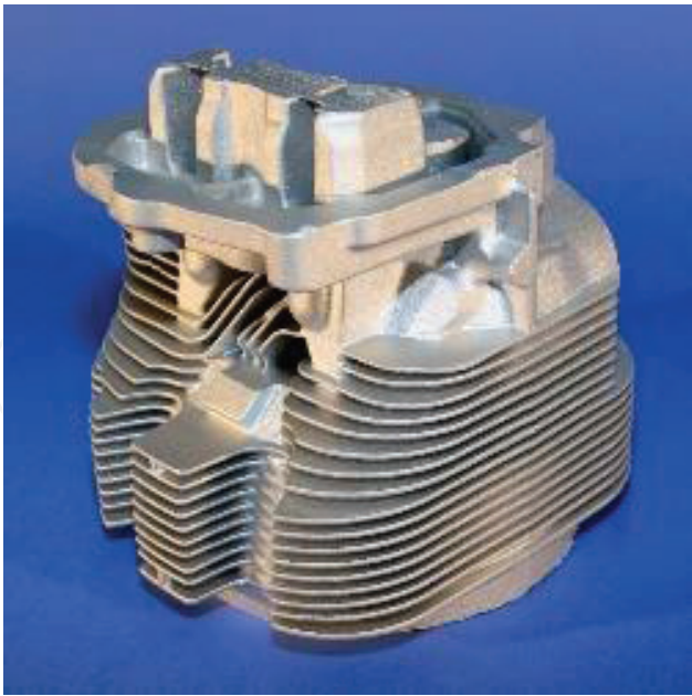
Figure 7. An air-cooled cylinder head cast in Al-8Ce alloy.
