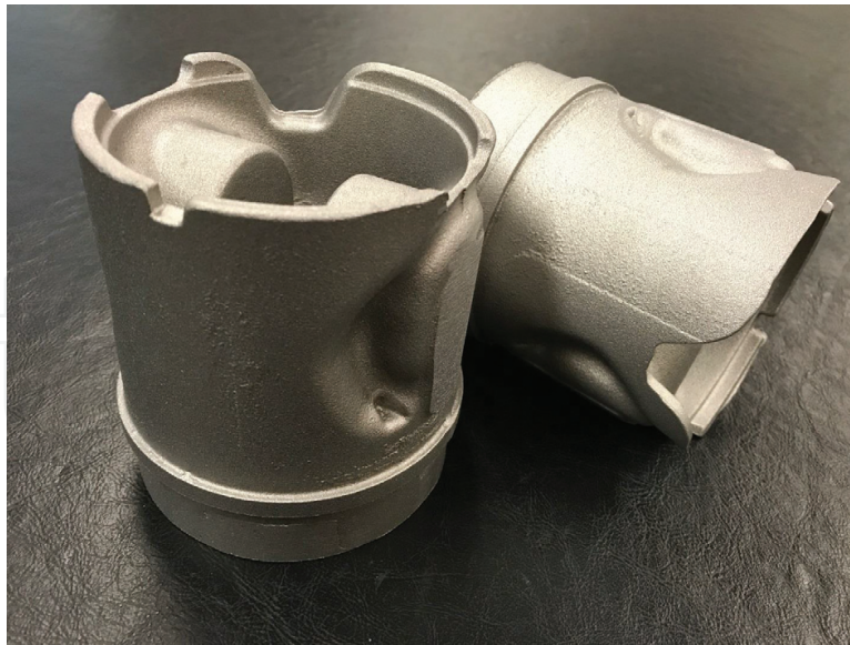
Figure 10. High performance pistons produced from various formulations of Al-Ce alloys.
