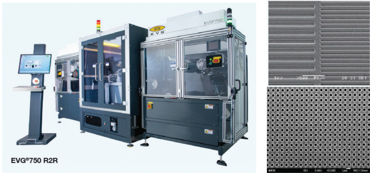
Figure 13. Photo of the EVG750 ® R2R hot embossing system, imprinted, SEM image of 10 μm and 30 μm microfluidic structures replicated into PMMA, 500 nm holes replicated into PMMA [31].
