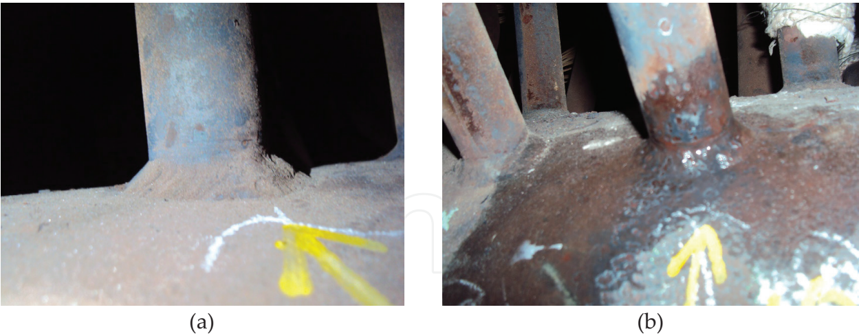
Figure 4. Appearance of tube failure at Row 3: (a) Tube 8 and (b) Tube 18.
