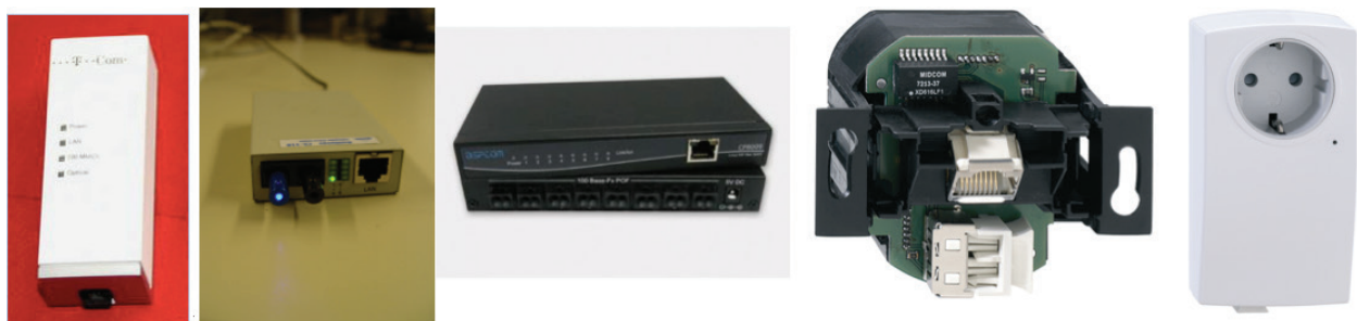
Figure 5. Tested media converter: Speedport, Diemount, BSPCOM, Rutenbeck and Homefibre.
