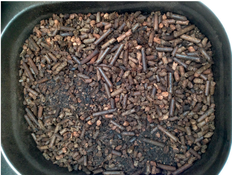
Figure 11. Photo of pelletized digestate—fuel for gasification reactor.
