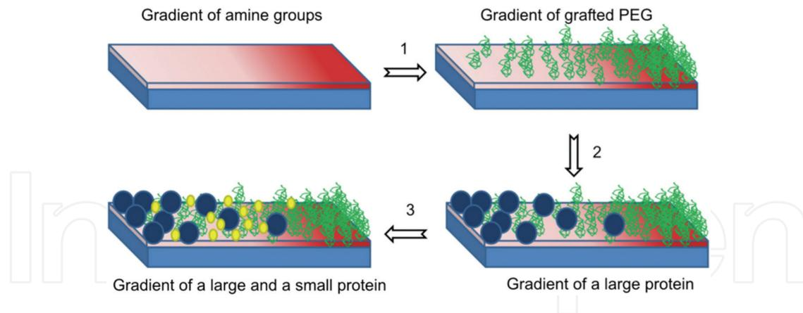
**Figure 5.** Schematic representation of the creation of two-protein gradient. Step 1. PEG grafting on the amine plasma polymer gradient to generate a PEG density gradient. Step 2. Large proteins adsorption. Step 3. Small protein adsorption.
