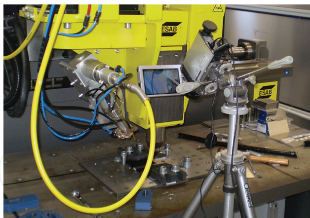
Figure 4. Thermographic experimental setup.
