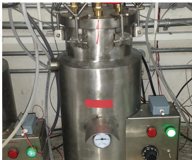
Figure 1. Laboratory-scale anaerobic reactor with pumped circulation.
