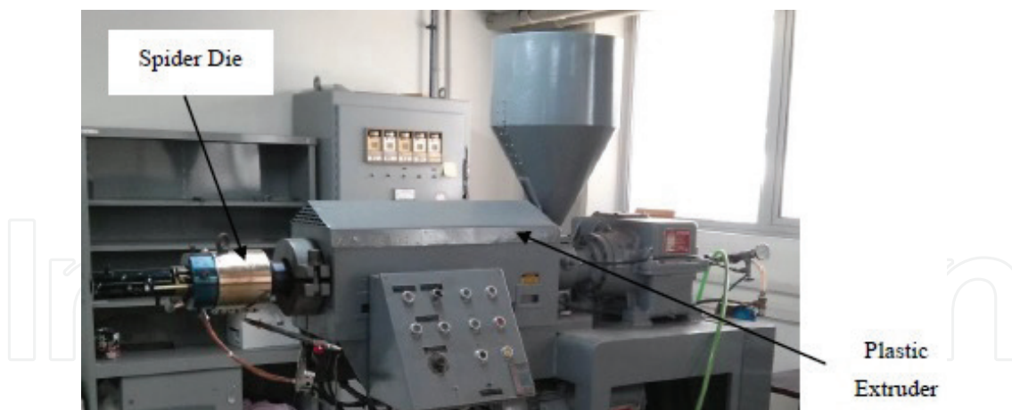
Figure 10. Johnson Plastics single-screw extruder together with the mounted extrusion die.
