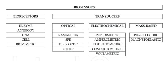
**Table 1.** Biosensors classification based on bioreceptor and transducer types.
