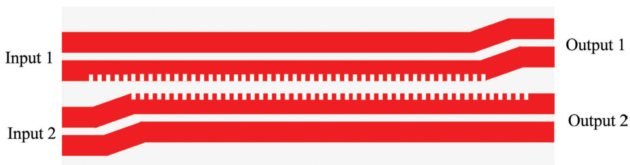
Figure 12. Schematic of a polarization-independent directional coupler based on slot waveguides with SWG structures.
