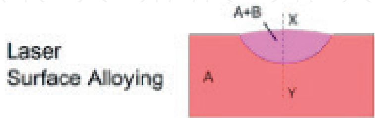
Figure 3. Schematic diagram displaying laser surface alloying [15].
