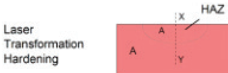
Figure 1. Schematic diagram showing the heat-affected zone of laser transformation hardening [10].
