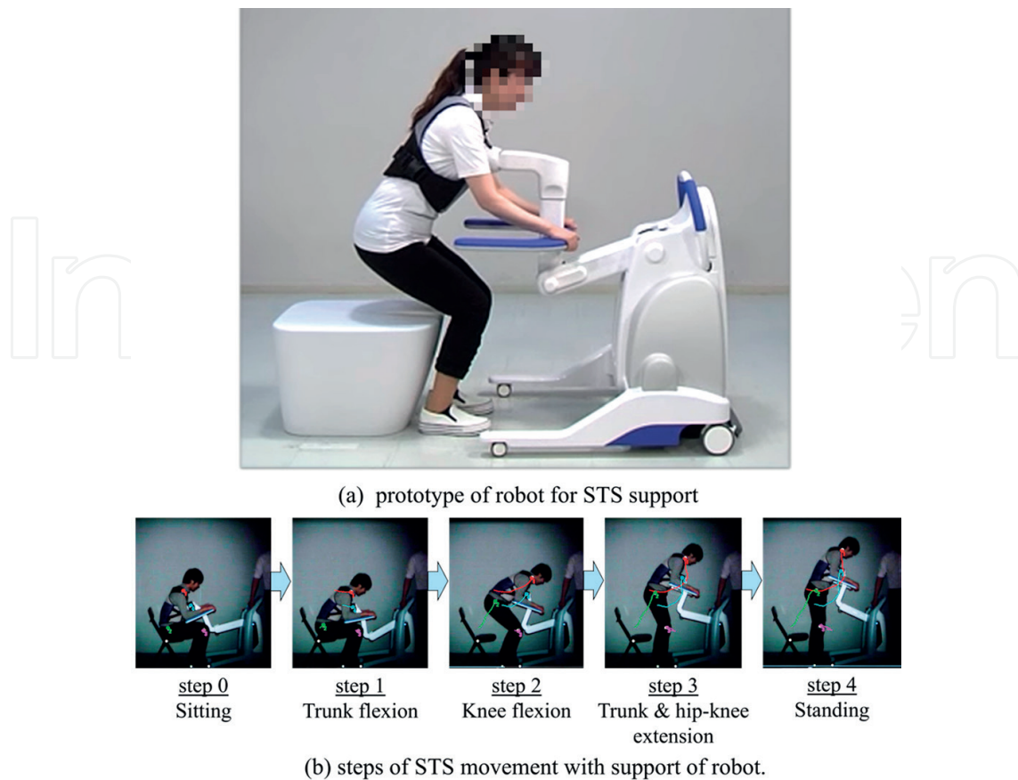
Figure 2. Overview of service robot. (a) A prototype service robot, complying with the ISO/TS 15066:2015 standard, with end-effect forces of 240 and 100 N in horizontal and vertical directions, respectively; (b) steps in robot-assisted STS movement, step (0) sitting still; step (1) trunk flexion; step (2) knee flexion; step (3) trunk and hip-knee extension; step (4) stabilization.
