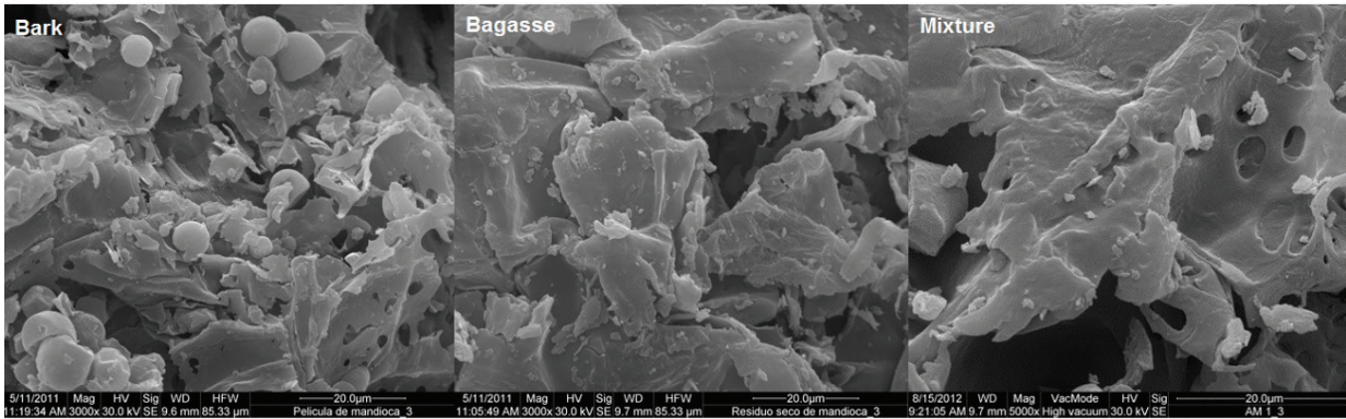
Figure 1. SEM of the adsorbents originating of cassava residues: barks (3000×) bagasse (3000×), and mixture of both fractions (5000×). Source: Refs. [9, 10].
