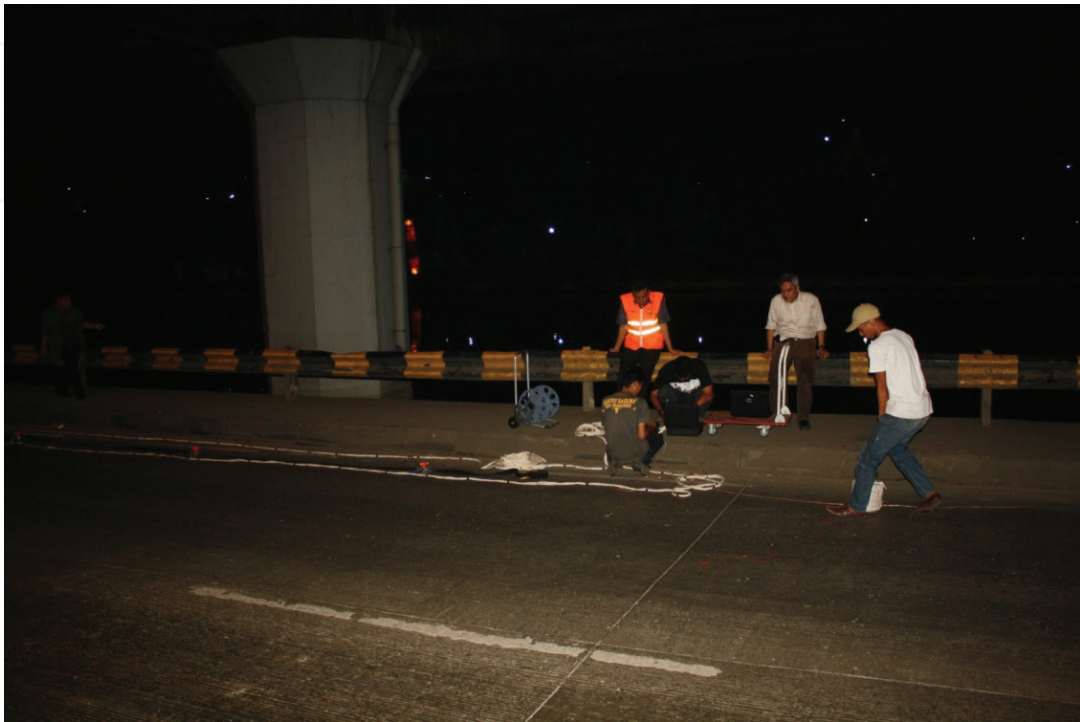
Figure 16. The weight drop used to generate vibration in repeat fashion (stacking method).
