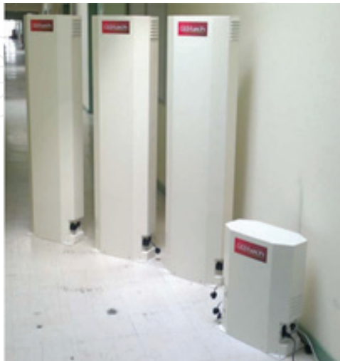
Figure 13. Photography of the RPM prototype (Katrina) developed by the CEA in the framework of the SECUR-ED project funded by the European Commission [30].
