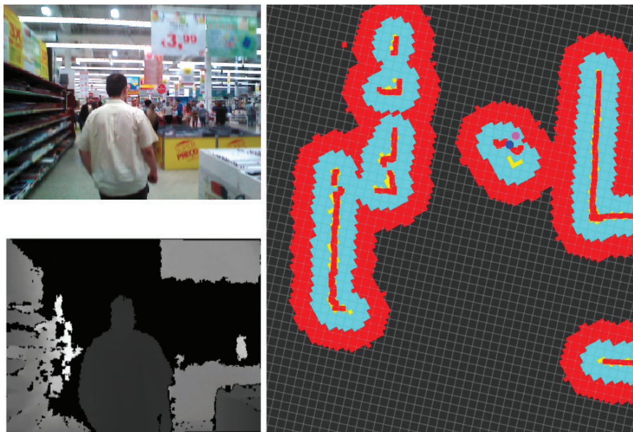
Figure 8. Tracking example where the person is visible both by the vision and by the 270° laser scanner. Purple dot in the map image corresponds to the person as localized by the image module, while the blue dot corresponds to the person as localized by the 270° laser scanner.
