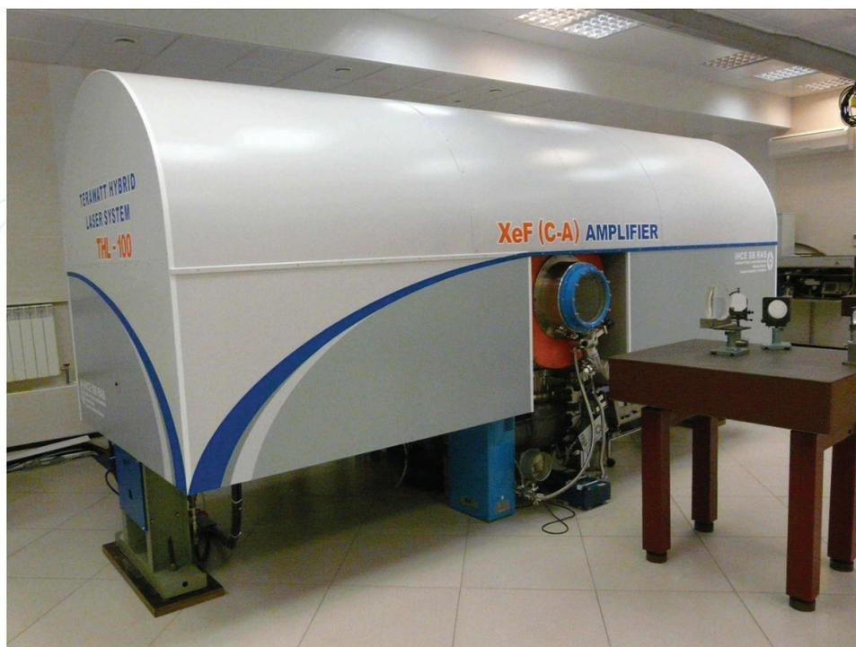
**Figure 12.** Photo of the XeF(C-A) amplifier.
