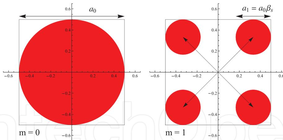
**Figure 4.** The rule of the deterministic mass-fractal construction.
