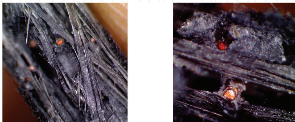
Figure 5. Tapering of conductive mesh (up to \times 200 magnification).
