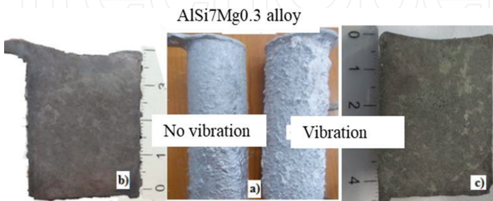
Figure 14. Photographs showing the roughness of the samples in AlSi7Mg0.3 alloy with and with no vibration (a), top part of the sample under vibration (b) and with no vibration (c) [10].
