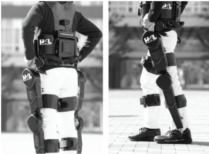
Figure 8. The HAL-5 type-C (hybrid assistive limb).
