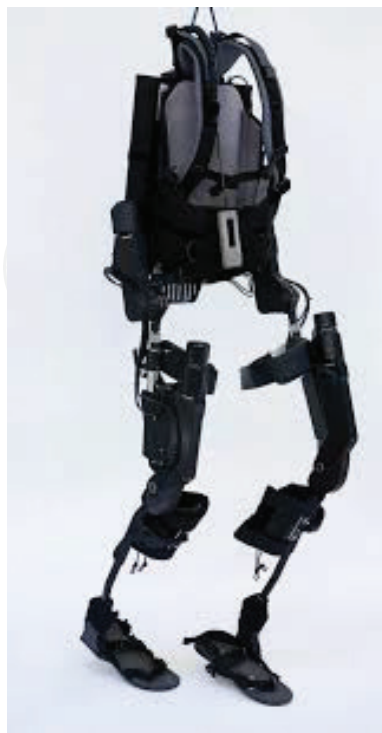
Figure 11. The eLEGS-powered orthosis (Berkeley Bionics).
