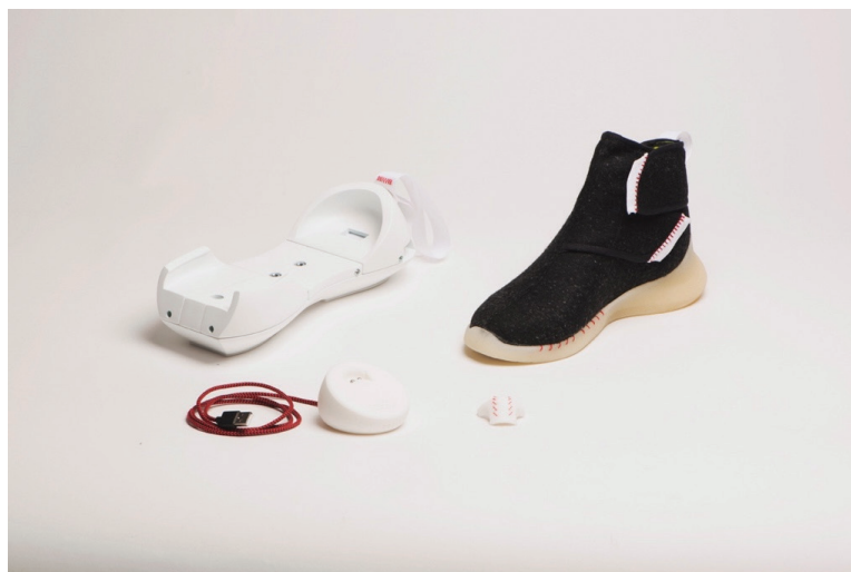
Figure 4. The physical game controller system: shoe, weighted sole, recharging dock, iMu sensors and cables.
