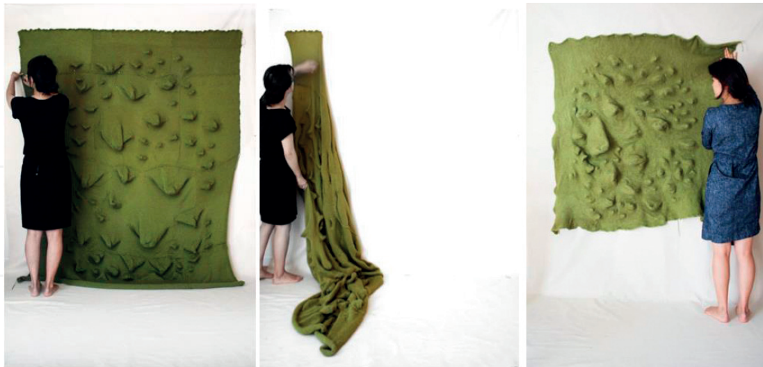
Figure 6. Felting process shrinks the woven wool textile by 30–40%. Felting transforms a woven knitted fabric into a seamless non-woven fabric.
