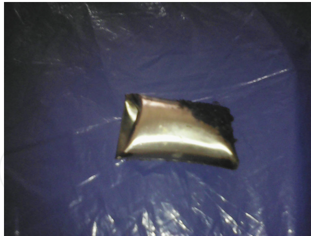
Figure 2. The mobile phone battery modified by the heat.
