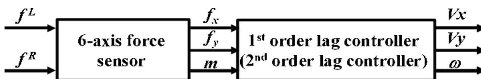
Fig. 27. Block diagram of the power-assist system
