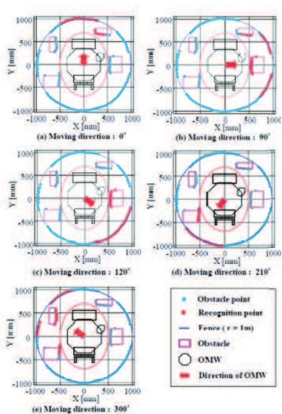
Fig. 13. Experimental results of environment recognition system
