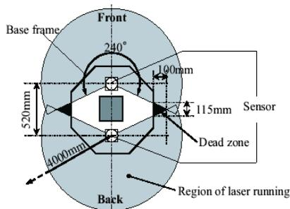
Fig. 8. Configuration of obstacle detection sensor (2)
