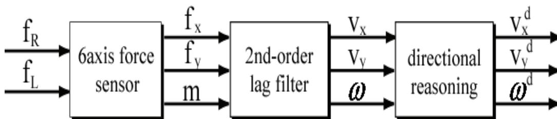
Fig. 37. Block diagram of the power assist system.
