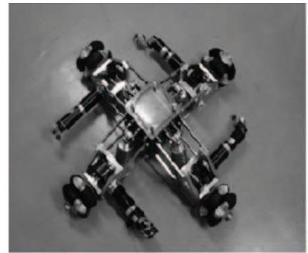
Fig. 3. Omni-wheels and motors
