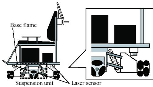
Fig. 7. Configuration of obstacle detection sensor (1)
