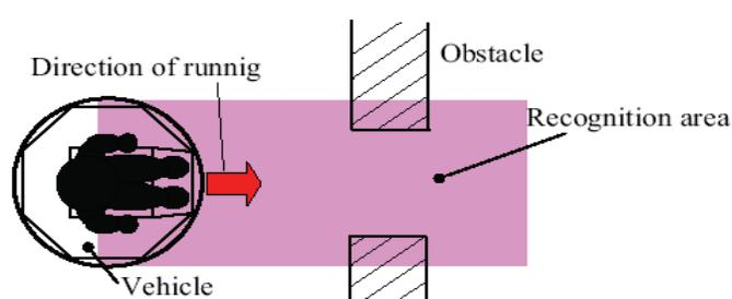
Fig. 5. Schematic diagram of environmental recognition and navigation
