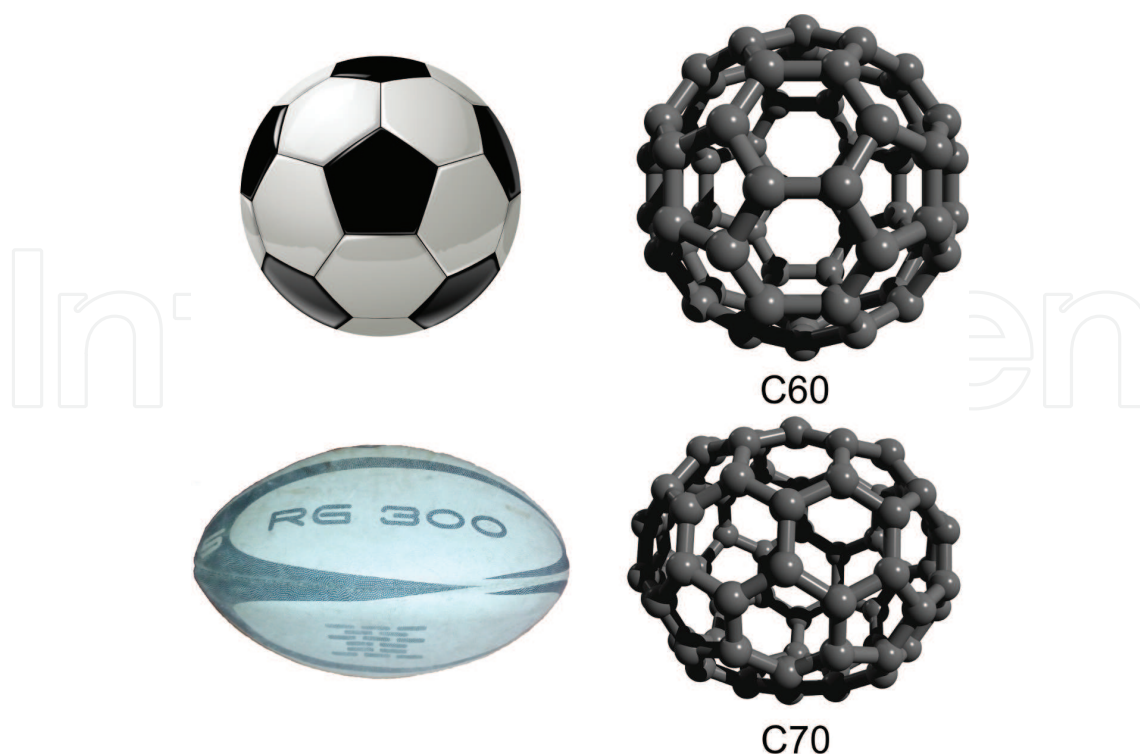
Figure 2. Comparison of C_{60} fullerene with a soccer ball and C_{70} with a rugby ball.
