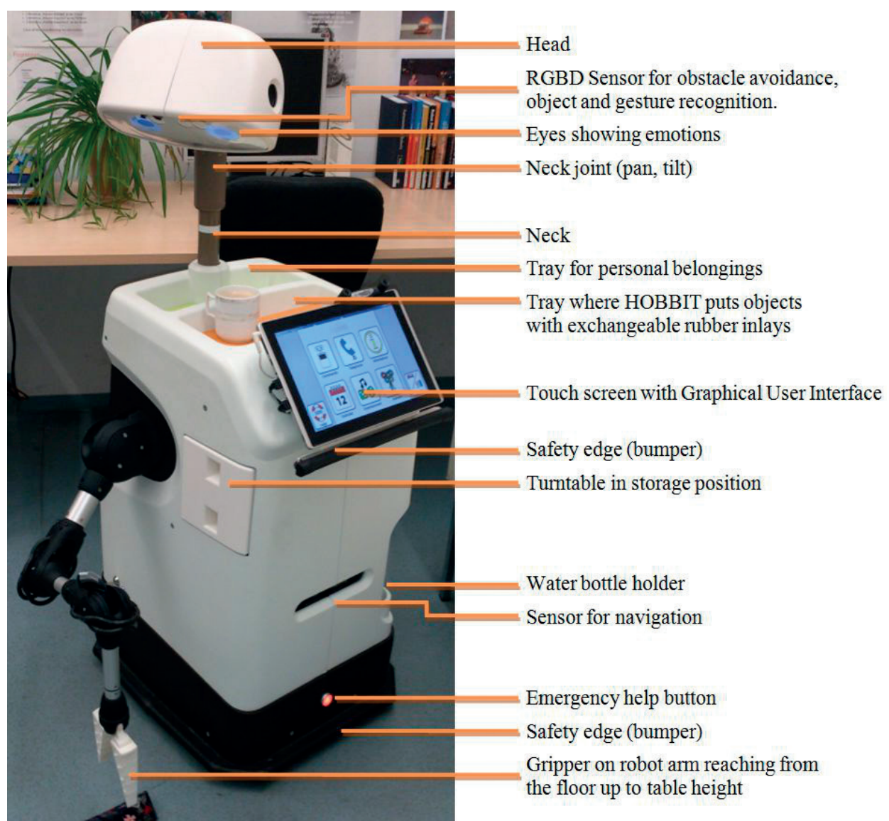
Figure 1. The service robot Hobbit designed to help older adults stay longer independent at home. Its primary functionality is coping with emergency situations, grasping objects from the floor or transporting objects to avoid falls and is a good collection of entertainment and physical and cognitive fitness functions.
