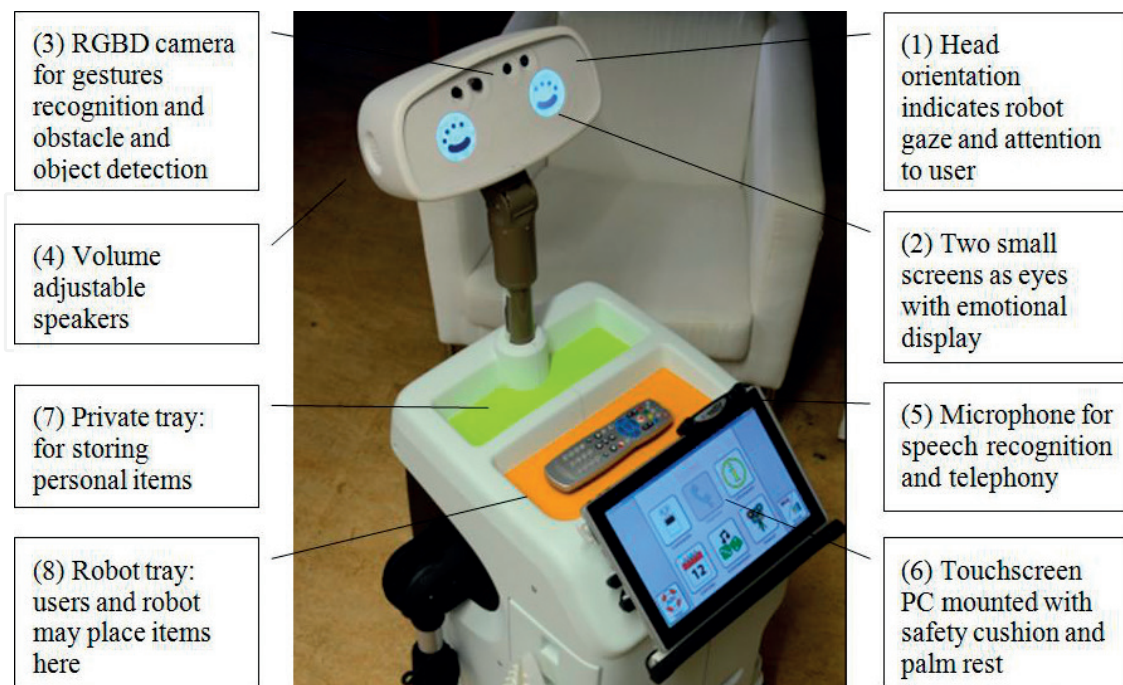
Figure 7. The upper body and the head of Hobbit. Also, depicted are the main components and functionalities.
