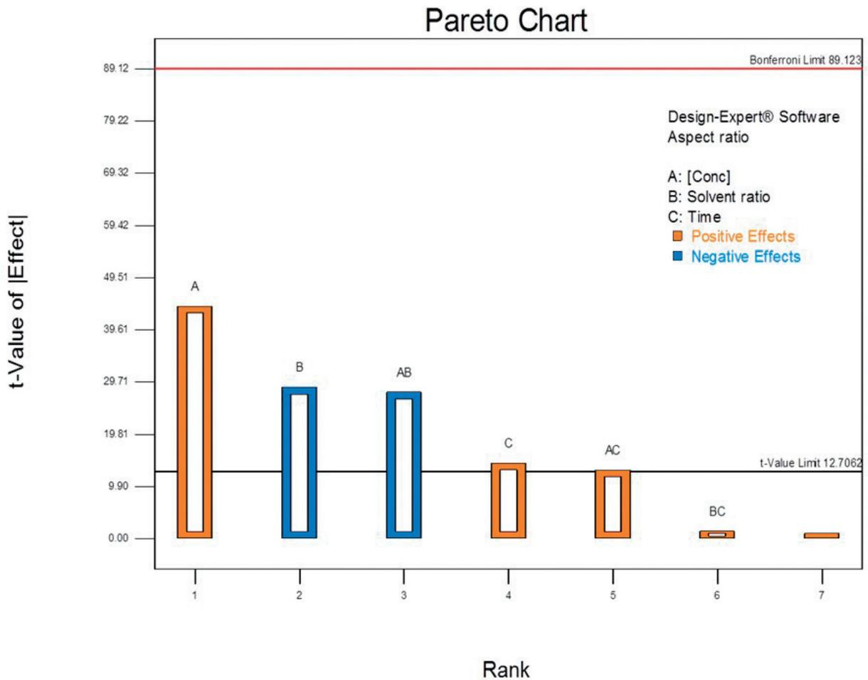
**Figure 2.** Estimated effects of factors on particle aspect ratio using factorial design.
