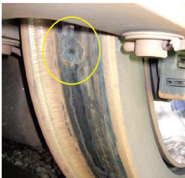
Figure 1. Photograph of a wheel flat formed by wheel-rail sliding [6].
