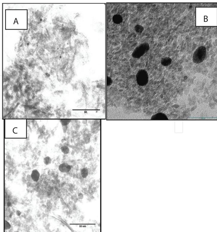
**Figure 5.** TEM images of Au/ $\gamma$ -Al<sub>2</sub>O<sub>3</sub> catalysts prepared by various reducing agents: (A) reduced with 5% H<sub>2</sub> (~4 nm); (B) reduced with THPC (~17 nm); and (C) reduced with PVA-citrate (~21 nm). Catalyst preparation details were outlined elsewhere [14].
