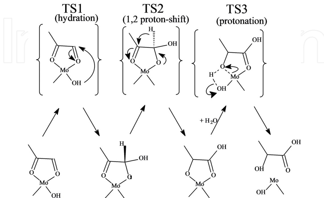
Figure 10. Possible Lewis acid-base pair dual site involved in the isomerisation of PA to LAC.
