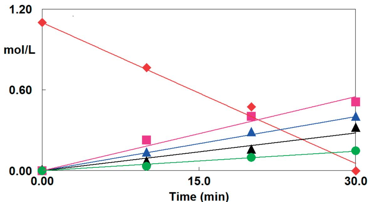
**Figure 8.** Comparison of computed and experimental data for glycerol oxidation assuming zero-order kinetics over  $\text{Au-MoO}_3/\gamma\text{-Al}_2\text{O}_3$  (top) and  $\text{Au}/\gamma\text{-Al}_2\text{O}_3$  (bottom); Glycerol (♦), glyceric acid (▲), FOP\* (▲), LAC (■), acetic acid (●).
