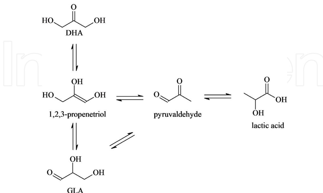
**Figure 9.** Proposed intermediates in the conversion of glycerol to LAC.
