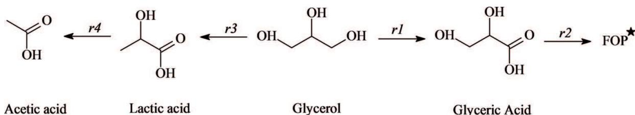
**Figure 7.** Reaction network used for the kinetic modelling of the glycerol oxidation. FOP\* = further oxidation products (tartronic, oxalic, glycolic and formic acids).
