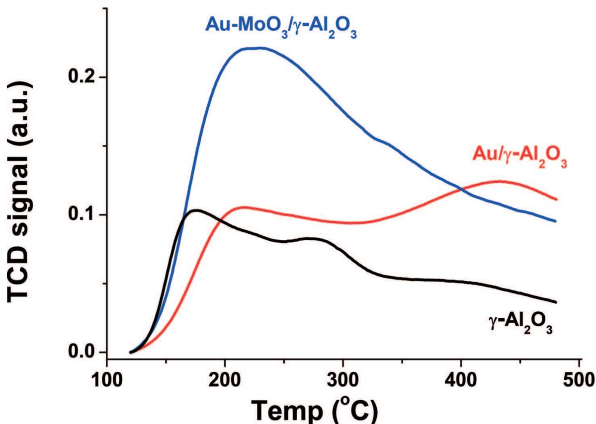
Figure 1. Qualitative analysis of the catalyst's acidity by the NH<sub>3</sub>-TPD method.
