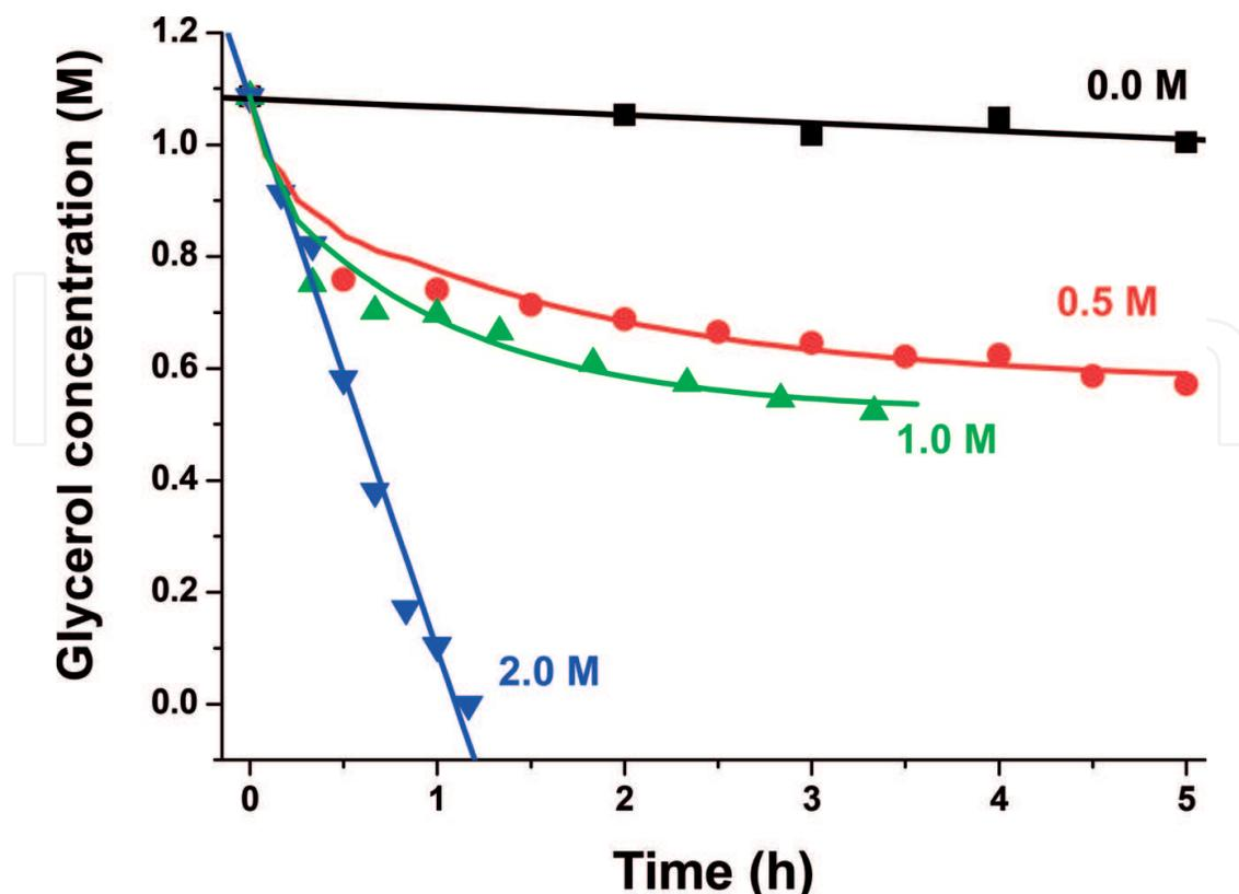
**Figure 2.** The effect of base concentration as a reaction initiator on glycerol oxidation using 0.5 g of 0.9-wt% Au/ $\gamma$ -Al<sub>2</sub>O<sub>3</sub> catalyst at 90°C and O<sub>2</sub> pressure of 8.5 bar.
