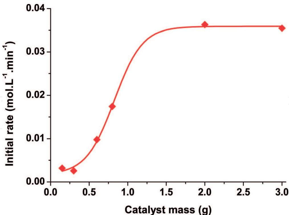
**Figure 3.** Initial rate as a function of catalyst mass for glycerol oxidation over 0.9-wt% Au/ $\gamma$ -Al<sub>2</sub>O<sub>3</sub> (106–150 m $\mu$ ): 1000 rpm, NaOH/glycerol = 2:1, at 60°C, under 8.5-bar O<sub>2</sub> pressure.
