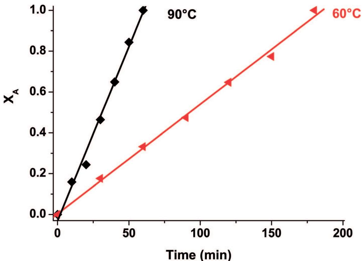
**Figure 4.** Conversion of glycerol over time by 0.9-wt% Au/ $\gamma$ -Al<sub>2</sub>O<sub>3</sub> (106–150 m $\mu$ ) catalyst; 1000 rpm, NaOH/glycerol = 2:1, at 60 and 90°C, under an O<sub>2</sub> pressure of 8.5 bar.
