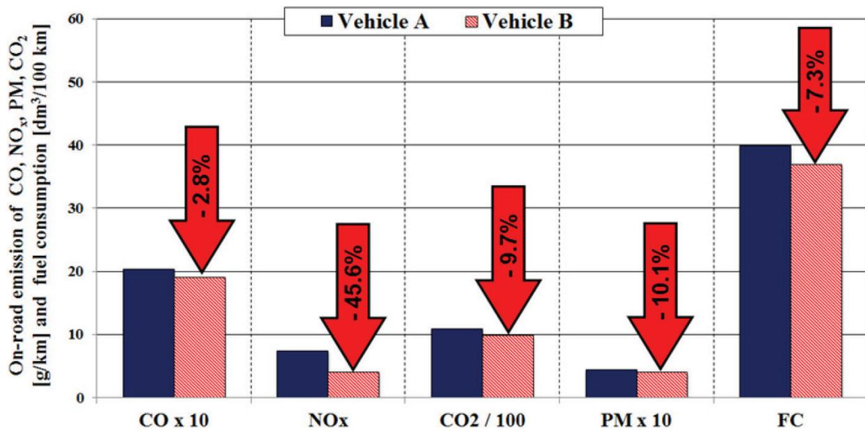
Figure 22. Comparison of the on-road emission of CO, NO<sub>x</sub>, CO<sub>2</sub>, PM and gas mileage of the tested vehicles.
