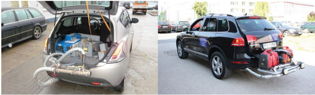
Figure 7. The tested objects ready for the on-road exhaust emissions tests.
