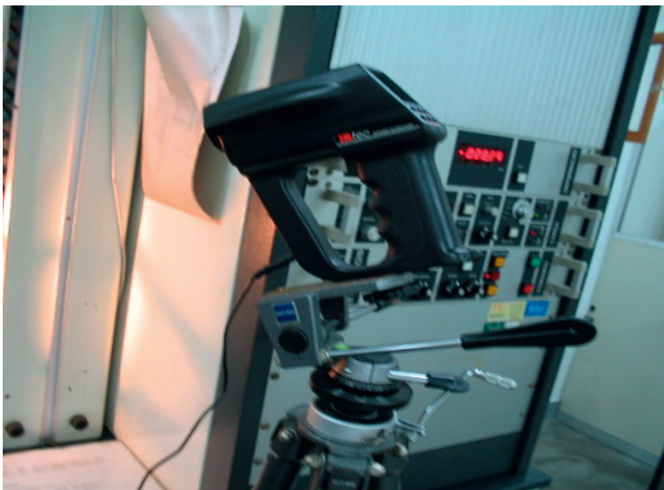
Figure 8. Maintenance of the system temperature with an optical pyrometer.
