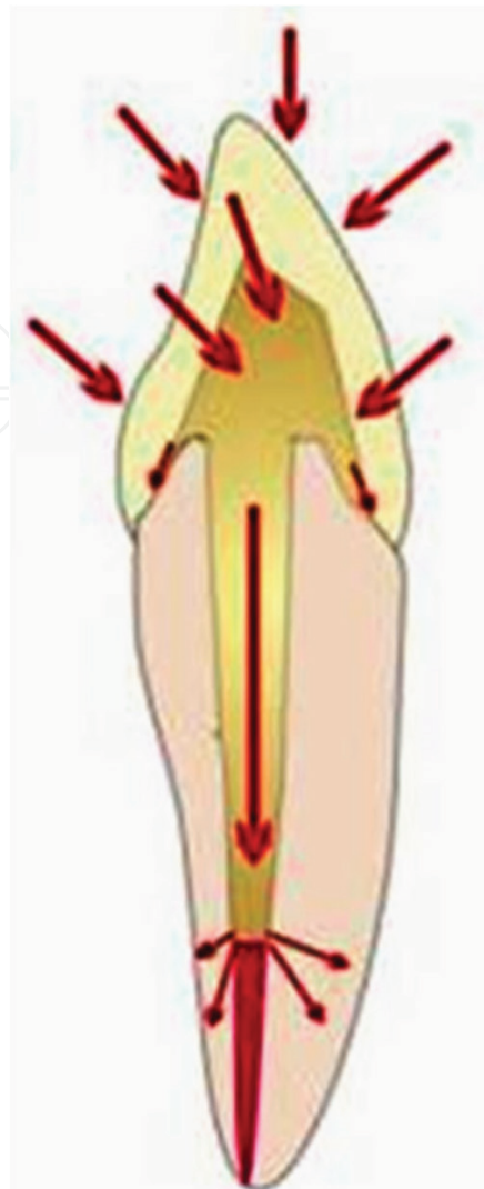
Figure 4. Stress concentration due to commercial dental post.
