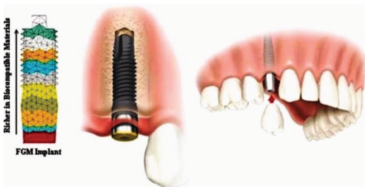
Figure 1. FGM dental implant with graded material composition.
