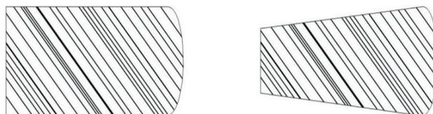
**Figure 9.** Top compression ring cross section.
