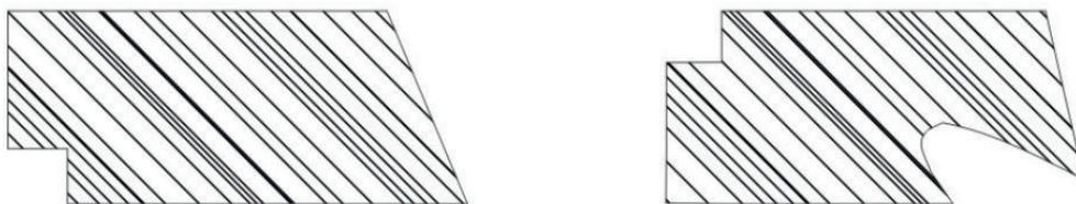
**Figure 10.** Second compression ring cross section.
