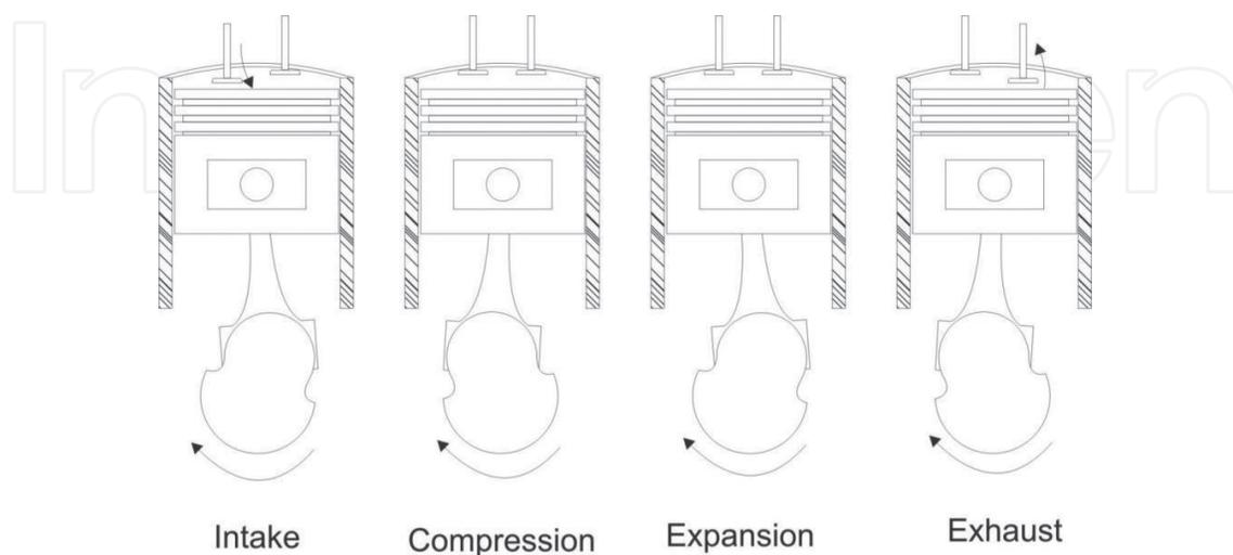
**Figure 2.** Four strokes for a complete engine cycle.
