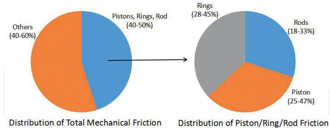
Figure 5. Power cylinder system friction power distribution.
