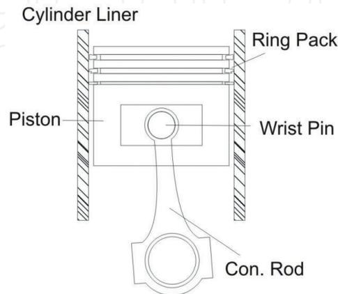
**Figure 1.** Power cylinder system.
