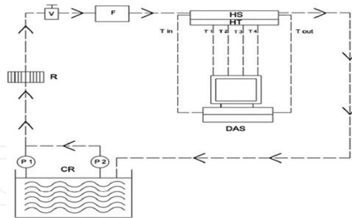
**Figure 3.** Schematic diagram of nanofluid flow through heat sink. CR is coolant reservoir, DAS is data acquisition system, F is flow meter, HS is heat sink, HT is heater, P is pump, R is radiator, T is thermocouple and V is valve in flow diagram.
