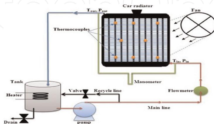
**Figure 1.** Flow diagram showing flow of nanofluid through radiator [11].
