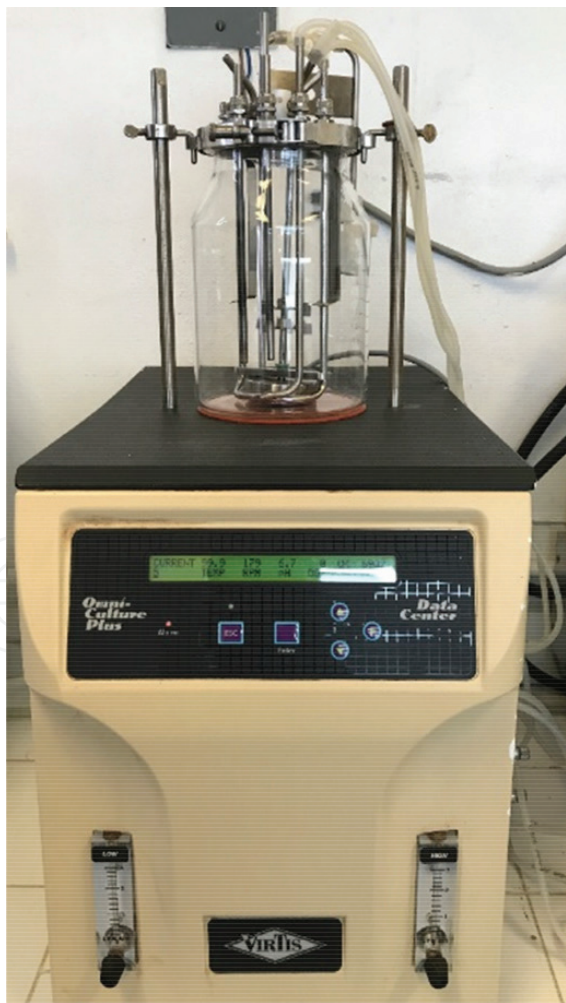
Figure 2. Chemostat Ommi Culture Plus (Virtis) used for fermentation experimental process.
