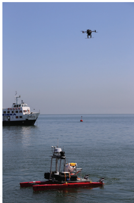
Figure 6. Rotary wing unmanned aircraft providing victim's location to ROAZ II (source: ICARUS).
