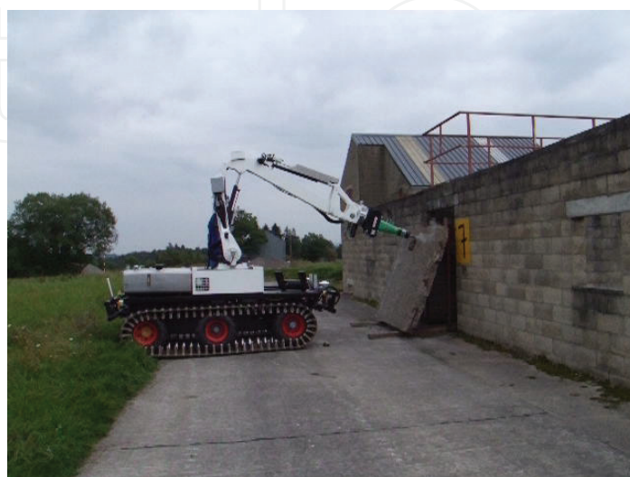
Figure 16. The LUGV uses its jackhammer to breach through a concrete plate (Source: ICARUS).
