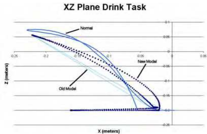
Fig. 10. XZ plane data of (from top to bottom) the drink task on ADLER. The data collected in normal mode is represented by a thick solid line, the data collected when using the old model is represented by a thin solid line (cyan), and the data collected when using the new model is represented by a dotted line.
